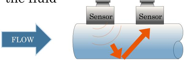
• Fluid must not contain high concentration of particles or bubbles
